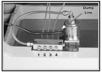
Figure 47. Oil pump and reservoir.
